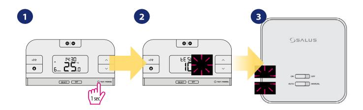
Press TEST / PAIRING button to check the connection with the receiver.
