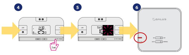
Press and hold TEST / PAIRING button for 3 seconds.
