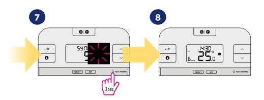
Press and hold TEST / PAIRING button for 3 seconds to end pairing process.
