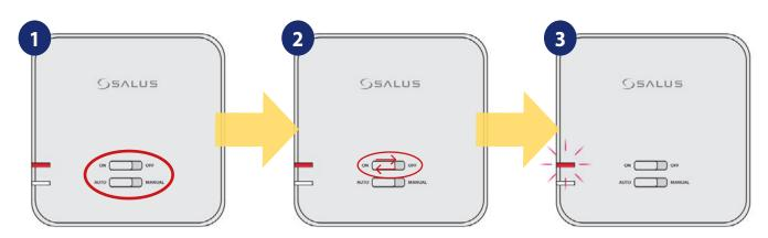
If you want to re-pair the devices with each other, make sure that the receiver is disconnected from the power supply and the switches on it are in the AUTO and ON positions. Then connect the receiver to the power supply and wait for the red diode to glow continuously.
