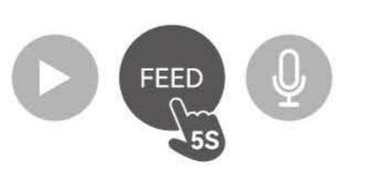
O Long press for 6 seconds to make a "dingdong" sound. Restart after restoring the factory settings (about 5 seconds), restart (the red indicator light goes out, the blue indicator light is normally on for about 15~18 seconds, and then the indicator light flashes slowly in the distribution network mode). Then, the feeder is reset and restarted.
