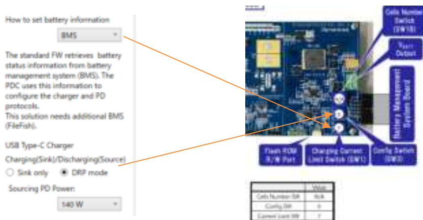
Figure 2-4 The Field E and the EVB setting vs “BMS” configuration
