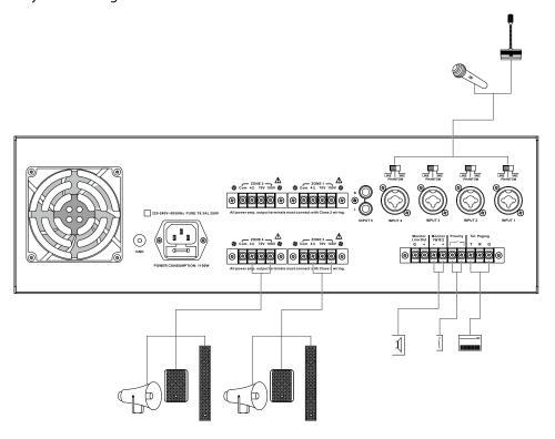
Finally check all cable connections for tightness and reattach the terminal screw strip covers to the device.
