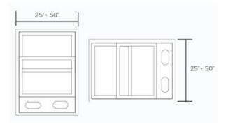
The window installation kit allows you to install the air conditioner in most vertical sliding windows 25" to 50" wide, or horizontal-sliding windows from 18" to 50" high.
