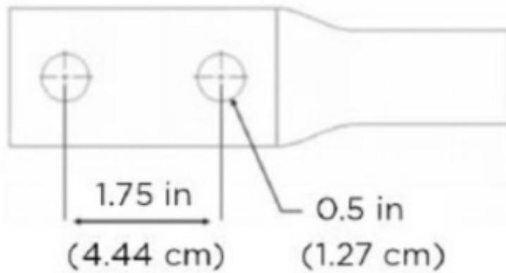
Figure 58: Bus Bar Dimensions - 1
