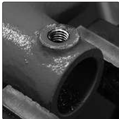
4.6 Thread is repaired and ready to use.
