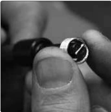
4.3 Load thread insert into installation tool.
