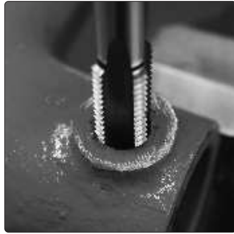
4.2 Tap drilled hole using screw tap provided.
