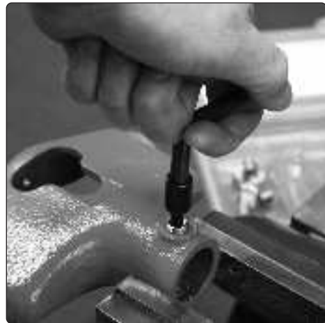
4.4 Screw insert into threaded hole.
