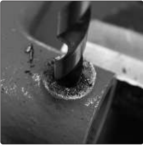
4.1 Drill out the damaged thread using the correctly sized twist drill bit provided.
