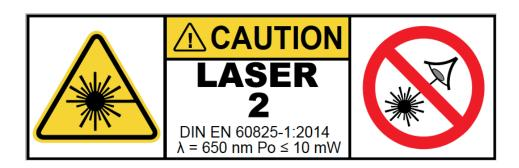
Operating and safety instructions for the operation of cross lasers for heat presses (laser class 2)
