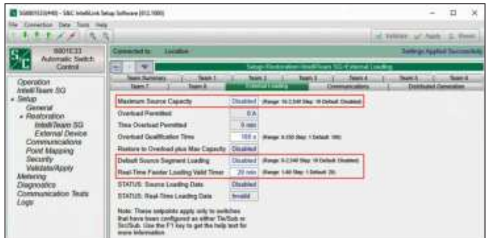
Figure 2. The Setup>Restoration>IntelliTeam SG>External Loading screen.
