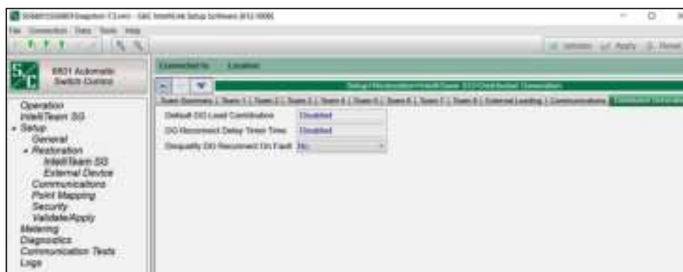
Figure 12. The Setup>Restoration>IntelliTeam SG>Distributed Generation screen.
