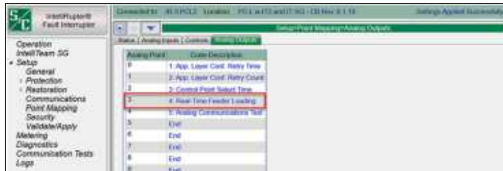
Figure 10. The Setup>Point Mapping>Analog Outputs screen.
