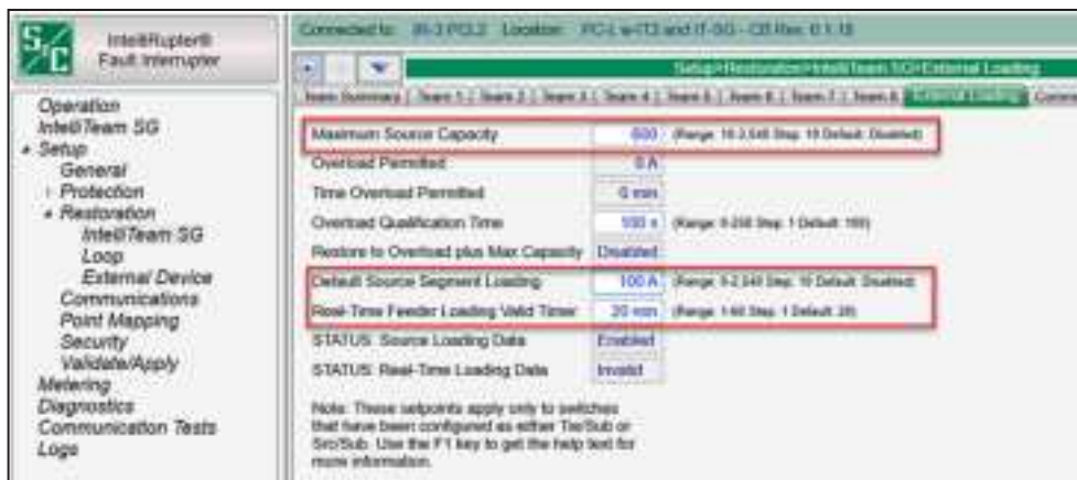
Figure 9. The Setup>Restoration>IntelliTeam SG>External Loading screen.
