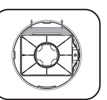
Remove the insulation sheet.
