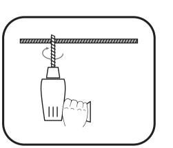
(This step is for installing on wood or cement, if installing on drywall, jump this step.) Drill a hole vertically on the wall. The hole diameter equal to the size of the expansion bolt.
