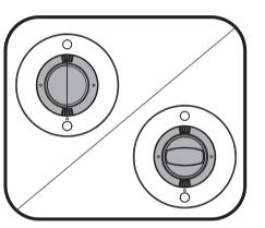
When the triangle icon on mask is 90 degree to the triangle icon on body, mask is locked.
