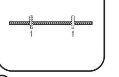
(This step is for installing on wood or cement, if installing on drywall, jump this step.) Insert the expansion bolt into the hole.
