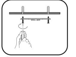
the screw vertically on the wall. For installing on wood or cement, lock the screw into expansion
