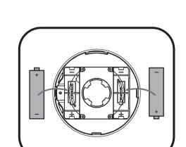
Install new battery. then reverse previous steps to finish the battery replacement. (Only use CR14505 for WOS3-PC)
