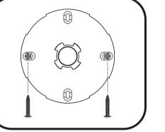
For installing on drywall, pass holes on the back plate. For installing on wood or cement, screw should pass the screws and align with the hole drilled
