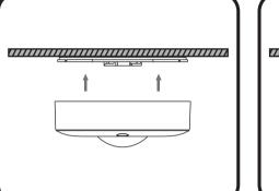
Align the device with back plate by positioning hole.
