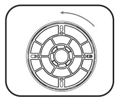
Counterclockwise rotation to separate the back plate
