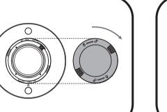
Put the ring into track, the Lock icon should be 10 degree to the triangle. Then clockwise rotate the ring.
