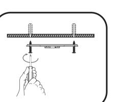
For installing on drywall, pass the screws through the installing
