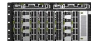
ACX7509 (Guardian) 9 slot (5RU) chassis 20x1-50GE 16x100GE 4x400GE (4.8T/J2C)
