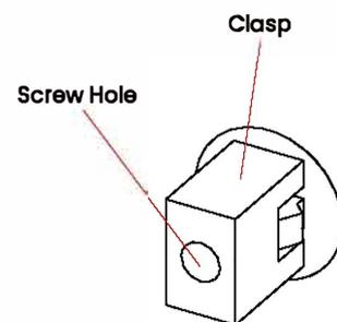
2. The grille shall align to the backside of the wall sleeve. The side where the guide track and slots are located should face towards the floor rather than the ceiling. The screw hole of the clasp shall align with the screw hole of the wall sleeve. Attach the grille to the wall sleeve from the outside of the sleeve, then install 6 screws from the inside of the sleeve to secure the grille to the sleeve.
