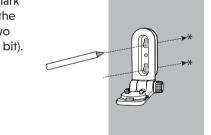
wall and then use a pencil to mark two holes in parallel. Remove the wall mount bracket and drill two holes in the wall (7/32 inch drill bit).
