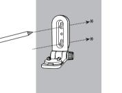
to step 3. If you drill the holes into an object other than a stud, insert the wall anchors into the holes. Tap gently on the ends with a hammer until the wall anchors
