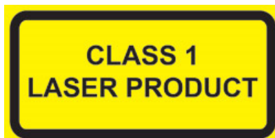
Figure 24. Label for Class 1 laser products
