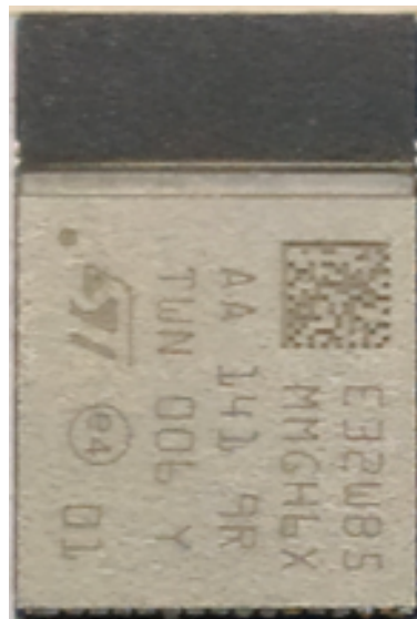
Figure 16. STM32WB5MMG RF module
