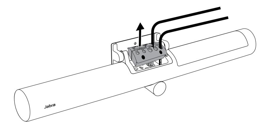
Attach the video bar to the Table Stand. Screws are not required.
