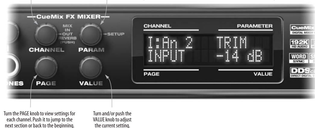
Figure 6-3: The 828mk3 front panel controls.
