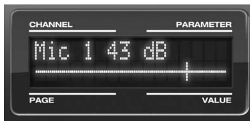
Figure 4-4: The LCD gives you feedback as you turn the TRIM knobs for the two mic/guitar inputs.
