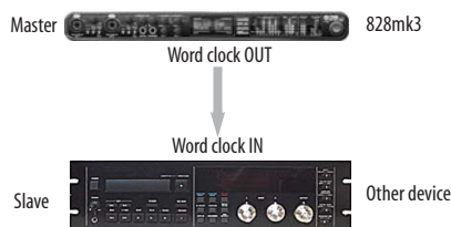
Figure 4-19: Slaving another digital audio device to the 828mk3 via word clock. For the 828mk3 clock source, choose any source besides word clock, as it is not advisable to chain word clock.
