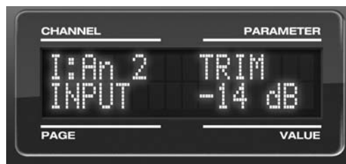
Figure 4-7: Setting the input trim for a TRS analog input pair.
