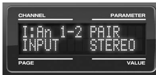
Figure 4-6: The settings for analog inputs 1 and 2 (as a pair).
