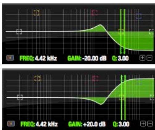
Figure 11-19: Overshoot when high shelf cut and boost is applied.
