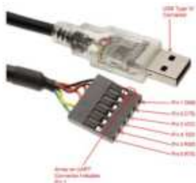
Figure 4: USB to Serial Pinout
