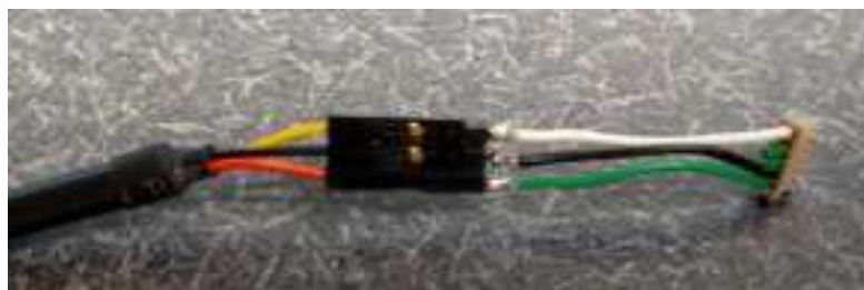
Figure 2: USB TO TTL UART Connector
