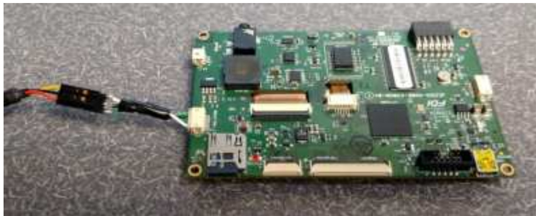
Figure 5: Connecting to the TTL UART
