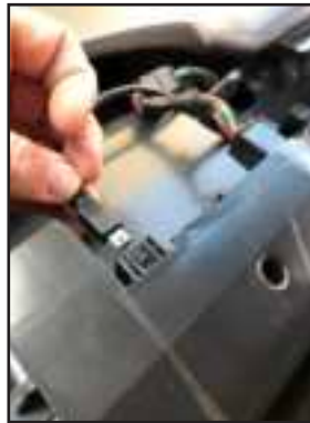
ACPGM-80N LVDS video cable plugs behind radio
