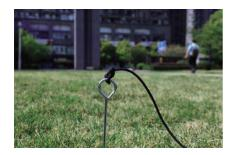
6. Insert the frame rod into the ground, the position should be at the end of "+" shape. Do not forget to across the metal ring when you insert the sliver nail into ground.
