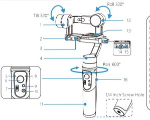
1 Tilt Motor 2 Thumb Screw 1 3.Mini USB (camera control) 4 Pan Motor 5.Bluetooth Light 6.Joystick 7.Slider 8.Mode Light 9 Mode Button 10.ON/OFF (Shutter Button) 11. Handle (Battery inside) 12 Roll Motor 13 Quick Release Plate 14 Thumb Screw 2 15. Ouick Release Plate Bolt 16.Power Indicator Light
