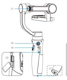
17.Thumb Screw 3 18.1/4 Inch Screw Hole 1 19.Trigger Button 20.USB Port 21.1/4 Inch Screw Hole 2
