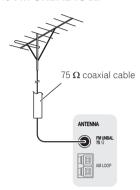
To improve AM reception, connect a 5 m to 6 m (16 ft. to 20 ft.) length of vinyl-coated wire to the  $AM\ LOOP$  terminals without disconnecting the supplied AM loop antenna.
