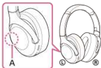
A: Location of the built-in antenna
