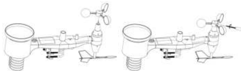
Figure 4: Wind Speed Cup Installation
