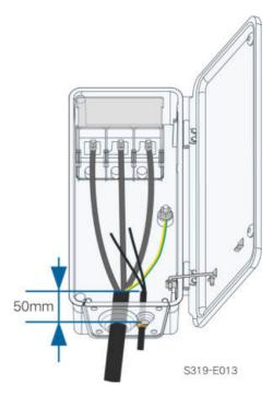
step 4 Stack the OT terminals on the OT/DT terminal of the AC cables, and fix the cables to corresponding terminals.
