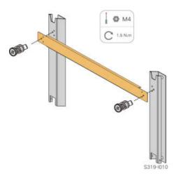
step 2 Level the assembled mounting-bracket by using the level, and mark the positions for drilling holes on the installation site.
