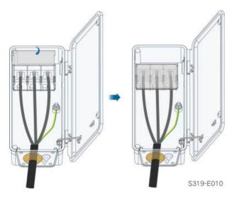
step 9 Remove the limit rod and place it in place. Close the junction block and tighten the two screws on its front cover with the hexagon socket wrench provided.
