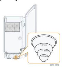
step 3 Lead the cable with the protective layer removed through the sealing ring. Retain 50mm of cable with the protective layer in the AC junction box.
