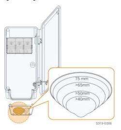
step 5 Lead the cable with the protective layer removed through the sealing ring and fix the screws on the bottom sealing plate.
