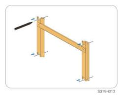
step 3 Drill the holes by using a hammer drill. Insert the expansion bolts into the holes and secure them with a rubber hammer. Fasten the nut with a wrench to expand the bolt. Remove the nut, spring washer, and flat washer, and store them properly.
