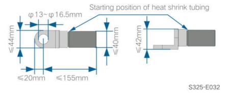
OT/DT Terminals of Phase Wire (Two Wires per Phase with Multi-core Cable)
