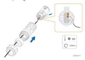
step 6 Pull cables outwards to confirm whether they are fastened firmly, then tighten the swivel nut with appropriate torque.
