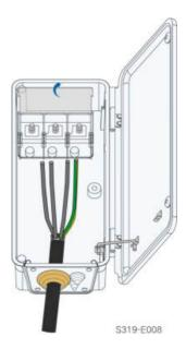
step 7 Fix cables with crimped OT/DT terminals to corresponding terminals.
