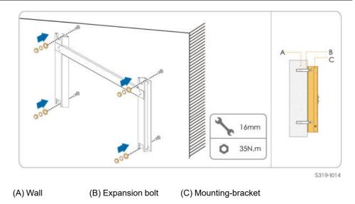
step 5 Fix the baffle plate to the wall with the expansion bolts.
