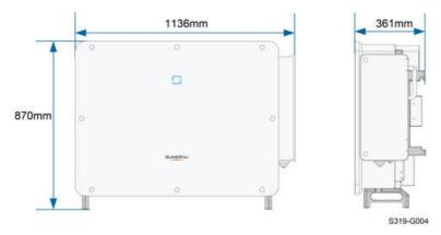
figure 2-3 Dimensions of the Inverter(in mm)
