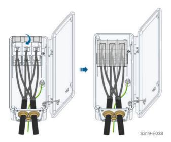
step 9 Remove the limit rod and place it in place. Close the junction block and tighten the two screws on its front cover with the hexagon socket wrench provided.
