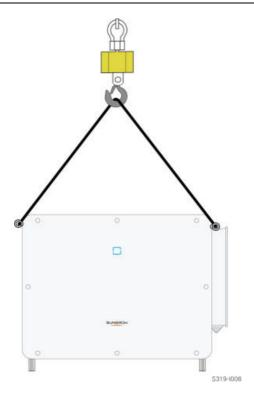
step 4 Remove the lifting rings and reassemble the sealing screws released in Step 1.
