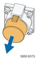
step 8 Insert the connector into the communication terminal.
