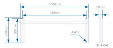
figure 4-1 Dimensions of mounting-bracket
