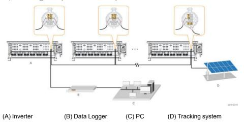
The length of the RS485 cable should be no longer than 1,200 m.
