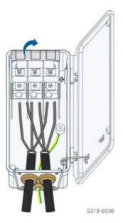
step 7  $\,$  Fix cables with crimped OT/DT terminals to corresponding terminals.
