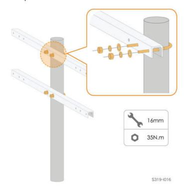
step 5 Use bolts to secure the pegboard to the U-beam.
