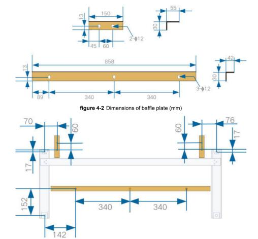
figure 4-3 Relative distance between baffle plate and mounting-bracket (mm)
