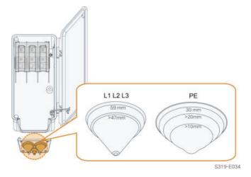
step 5 Lead the cable with the protective layer removed through the sealing ring and fix the screws on the bottom sealing plate.
