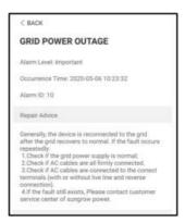
figure 7-8 Detailed Fault Alarm Information
