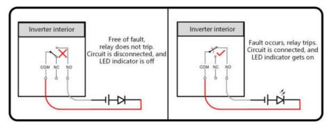
figure 5-8 Normal open contact
