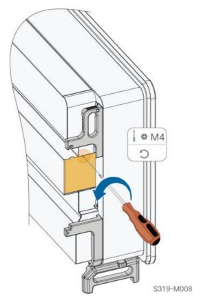
step 3 Press the tab of the latch hook, unplug the cable connection joint outwards, and loosen the screw on the fan holder.
