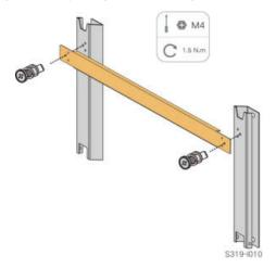
step 2 Place the assembled mounting-bracket onto the PV bracket with the distance between the mounting-bracket and the ground shown in the figure. Adjust the angle with a level and mark positions for drilling holes. Drill the holes by using a electric drill.
