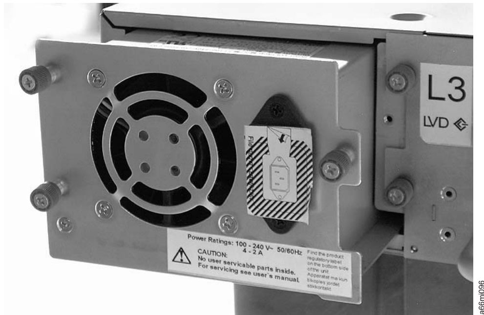
Figure 9-5. A power supply being removed from the library
