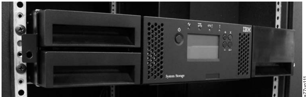
Figure 2-8. Sliding the 2U library into the rack
