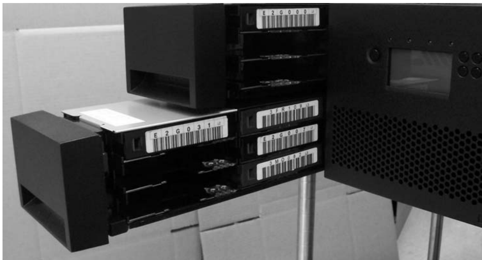
Figure 8-4. Left Magazines pulled out of the 4U Library
