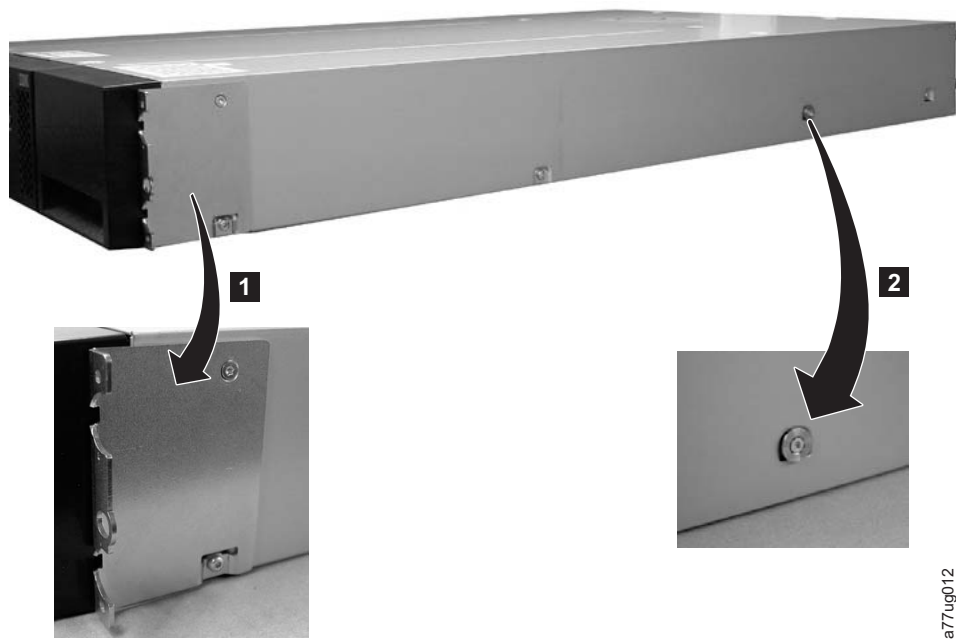
Figure 2-7. 2U library rack anchors and mounting brackets
