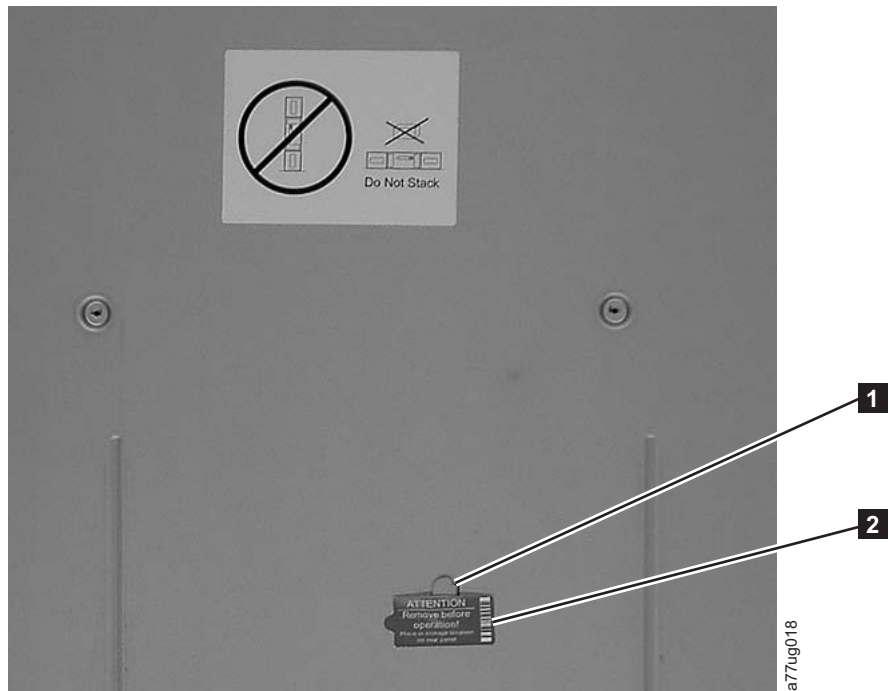
Figure 2-2. Shipping lock and label
