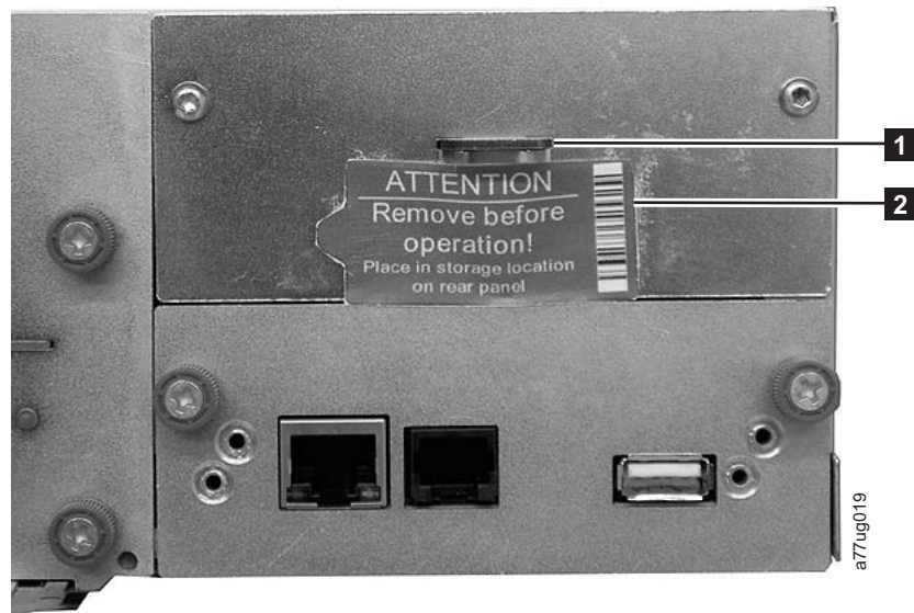
Figure 2-3. Library shipping lock and label storage location
