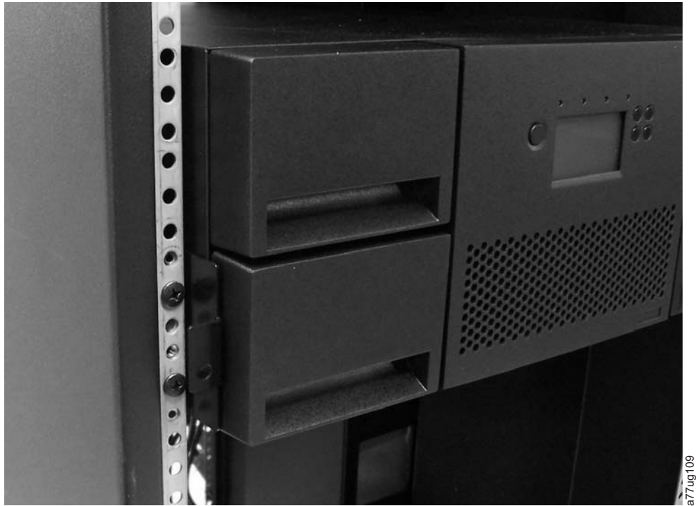
Figure 2-9. Sliding the 4U library into the rack
