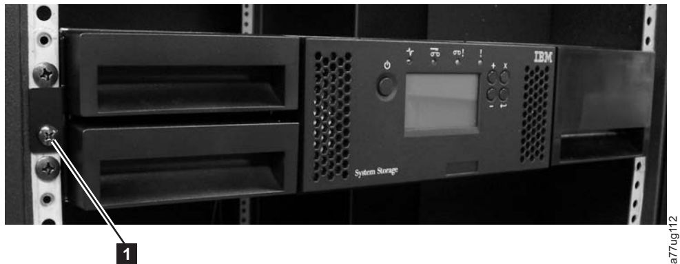
Figure 2-10. Securing the 2U library to the rack
