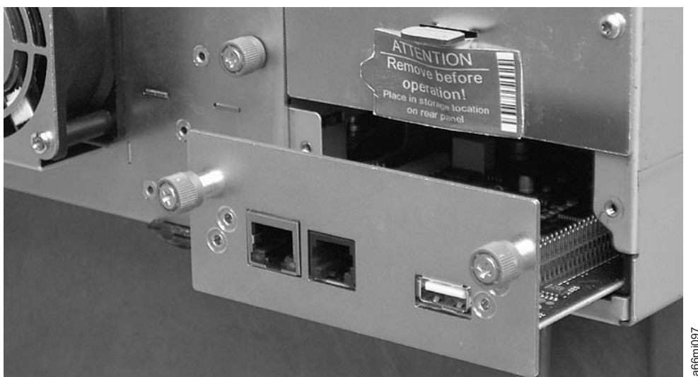
Figure 9-6. A Library Controller Card being removed from the library
