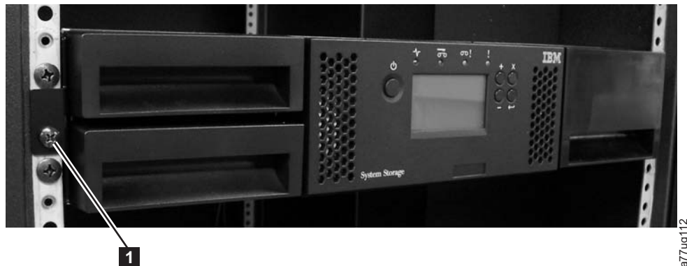
Figure 9-10. Removing the two screws anchoring the library to the rack
