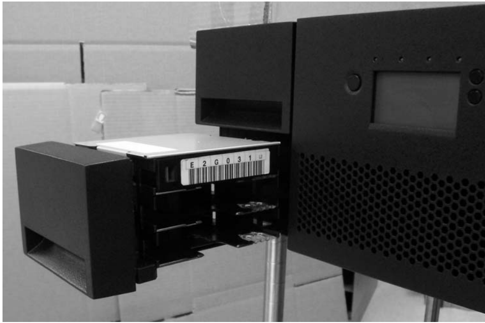
Figure 2-32. 4U library I/O Station in the lower left magazine
