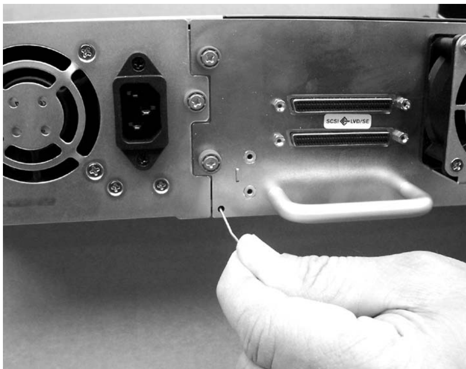
Figure 8-1. Access holes for the left magazine
