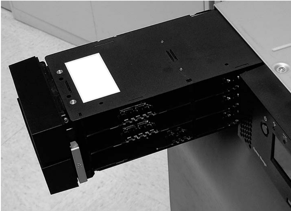
Figure 8-3. Left magazine pulled out of the 2U library
