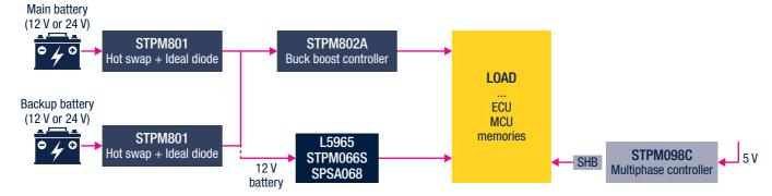
The whole portfolio has been designed to fulfill functional safety requirements as defined by Automotive Safety Integrity Level (ASIL).
