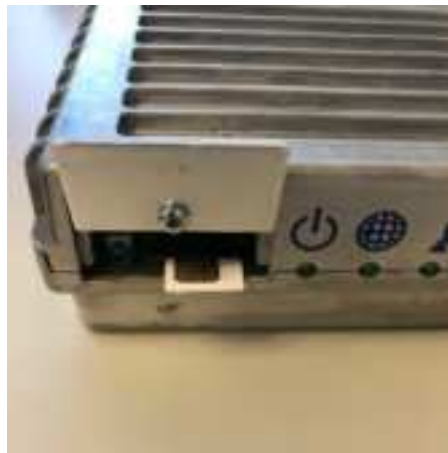
Figure 32: Installing the SIM card
