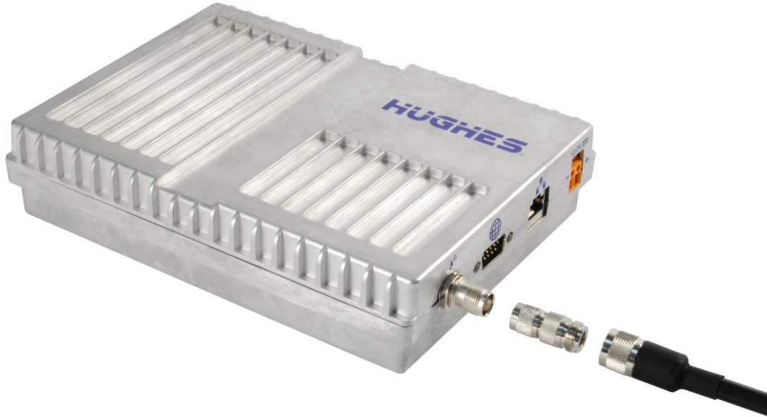
Figure 31: Connect cable to TNC connector on IDU
