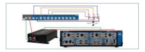
FIGURE 10. Setup with APx555.
