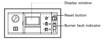
Control unit for weather-responsive operation with programming unit
