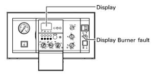
Control unit for weather-compensated mode with standard programming unit
