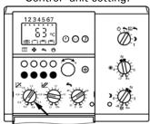
Setting of coding address "08" Slope setting range "08:00" = 0.2 to "08:15" = 2.6 (Change per step: 0.2) As delivered condition: "08:09" = 1.4.
