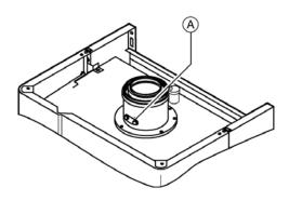
A Combustion air measuring point
