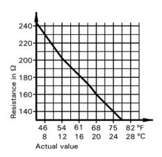
RS remote control Room temperature sensor (NTC) curve between terminal "9" and "13"
