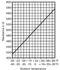
Check boiler temperature sensor
