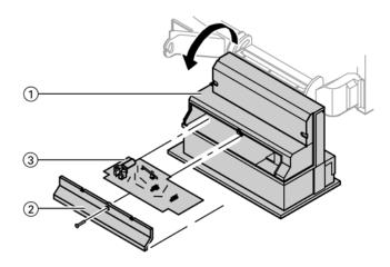
Before replacing circuit board VR20, record actual system addresses (in particular coding addresses 000, 0B8, 042, 045, 015, 017, 0A2) and their corresponding values, heating curves and DHW settings.
