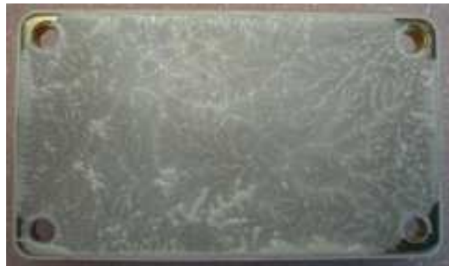
Picture 3: Grease on the module after disassembling
