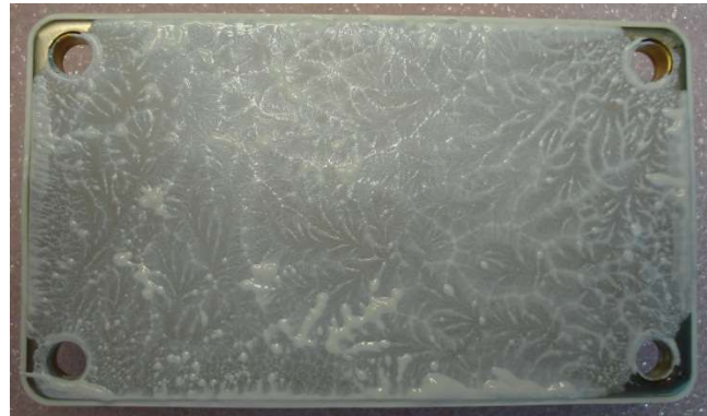
Picture 3: Grease on the module after disassembling
