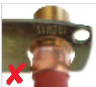
Fitting has been under crimped
