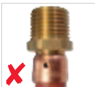
Witness hole not completely filled
