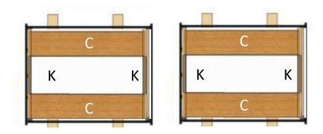
After all 2 boards and 16 spacers are installed, confirm that the frame, boards, and spacers remain stable on the support structures before proceeding to the next step.
