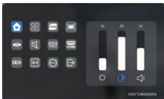
Luminance: Press the Up and Down keys to adjust the luminance.
