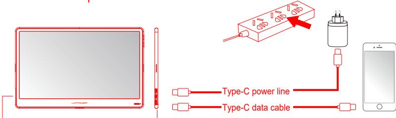
1. Connect the Type-C data cable to one of the Type-C ports of the machine and connect the other end to the mobile phone.
