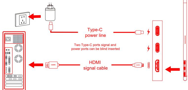
1. Connect the HDMI cable with the Mini-HDMI port of the product and the HDMI port of the PC.
