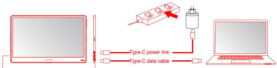
1. Connect one end of the Type-C data cable to one of the two Type-C ports of the machine and the other end to the Type-C signal port of the laptop.
