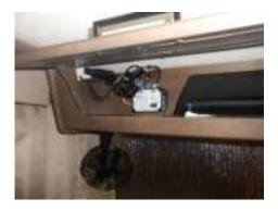
Location of bed slide out controller in storage small compartment at back of coach. Same location as the low point freshwater tank drain.
