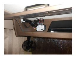
Location of bed slide out controller in storage small compartment at back of coach. Same location as the low point freshwater tank drain.
