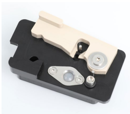
O-Ring tool with prepared new O-Ring
