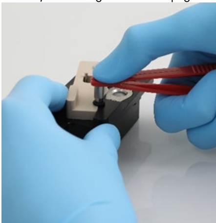
Press the peg down using the back end of the tweezers
