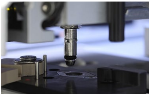
Check if the new O-Ring sits firmly
