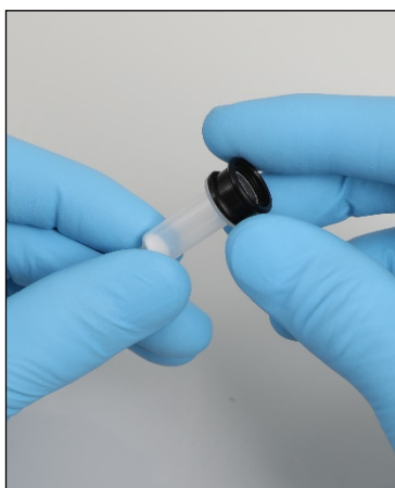
Mounting a spin column adapter ring.
