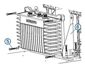
5 Align the chartplotter bail mount over the hole pattern that matches your bail mount, with the openings on the top of the bail mount facing the back of the base.
