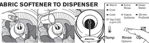
**IMPORTANT:** Fabric Softener option must be selected to ensure proper distribution at correct time in cycle.
