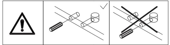
Insert wooden dowel(D) into board 3 at first, then attach board 26 and fix with screw(F) as shown.
