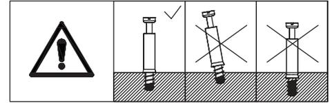
Insert quickfit screw(A) into board 25 at first, attach to board 3 with wooden dowel(D). Put cam lock(B) into board 3 and turn clockwise to tighten as shown.
