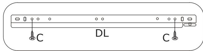
Fix runner (DL) and (DR) to board 16 and 18 respectively with screw (C).
