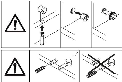
Insert wooden dowel(D) into board 5 at first, then the leg base to.
