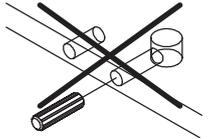
Insert wooden dowel(D) into board 2 at first, then attach board 26 and fix with screw(F) as shown.
