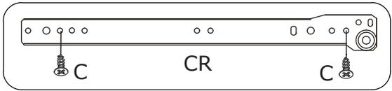
Fix slide rail(CR) to board 26 (assembled in board 3) with screw(C) as shown.
