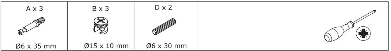
Insert quickfit screw (A) into board 10 at first, attach to board 2 with wooden dowel(D).
