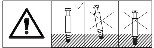
Insert quickfit screw(A) into corresponding holes in board 2 and 3 with a screwdriver as shown.
