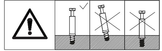
Attach board 6 to board 1 with screw(H)
