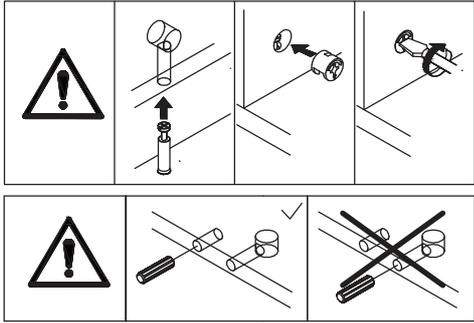
Insert wooden dowel(D) into board 3 and 25 at first, then attach board 8, 24 and 7. Put cam lock(B) into board 8, 24, 7 and turn clockwise to tighten as shown.
