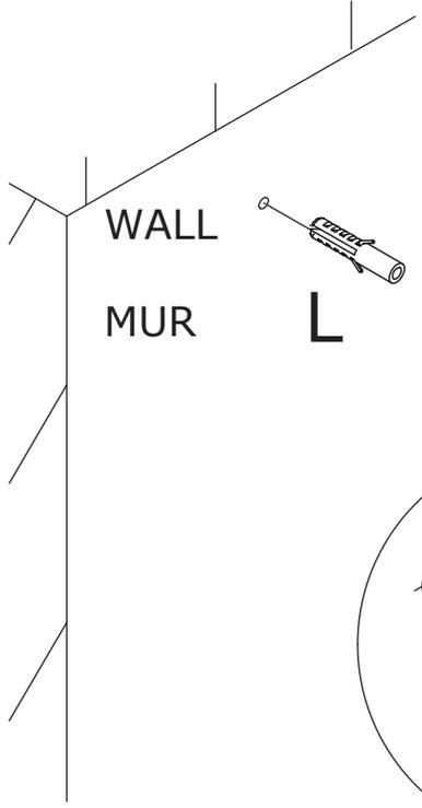
Install anti-tipping device as shown.
