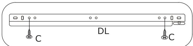
Fix runner (DL) and (DR) to board 16 and 18 respectively with screw (C).
