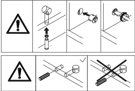
Insert wooden dowel(D) into board 2 and 10 at first, then attach to board 8, 24 and 7. Put cam lock(B) into board 8, 24, 7 and turn clockwise to tighten as shown.
