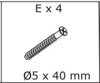
Attach board 5 to board 2 and 3 using wooden dowel(D), and fix with screw(E).
