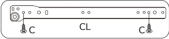
Fix slide rail(CL) to board 26 (assembled in board 2) with screw(C) as shown.
