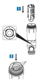
Install the filter assembly, taking care that when loading the screen assembly the four raised points on the screen assembly need to against the four grooves of the filter bottle, and install to the end.
