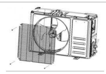
**1).** Unfix the screws on the front panel of the fan guard.
