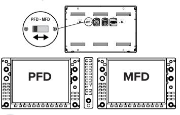
The 12VDC power supply must be disconnected for the change to be applied. Otherwise, the device will remain in the previous state.
