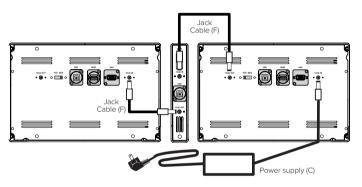
**4.** Connect the adequate power cable (D/E) for your country's nominal voltage to the power supply (C).
