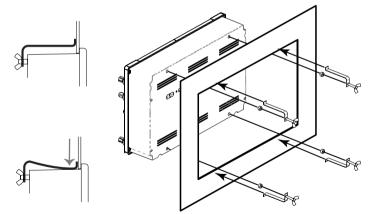
To mount the PFD/MFD to your custom flight panel from the back, your panel will need a cutout that matches the measurements depicted in the blueprint below. All measurements displayed are in millimeters.
