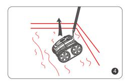
You can insert the included hook into a pool pole and lift the cleaner out of the pool.
