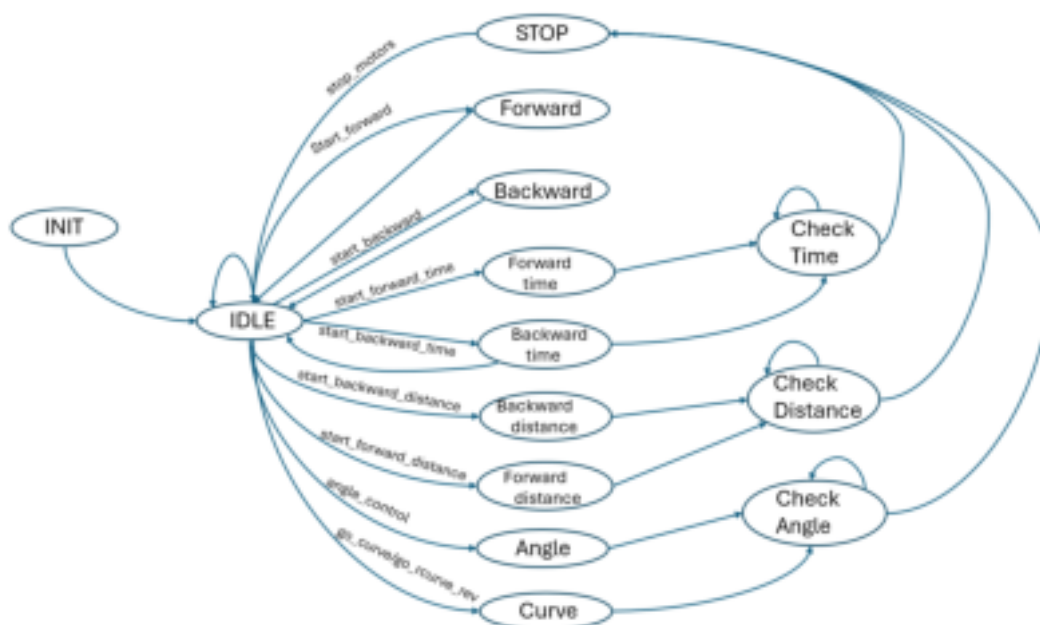
Figure 31. State Machine for STSW-ROBKIT1-2
