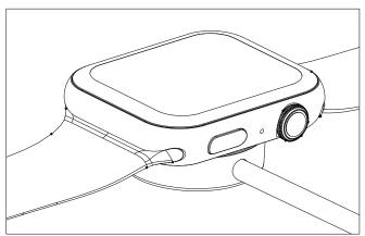
Charging Tips: To achieve maximum charging current and optimal magnetic attraction, please refer to the provided picture to align the charging dock with the center line of the button on the watch. This positioning ensures the best charging angle.
