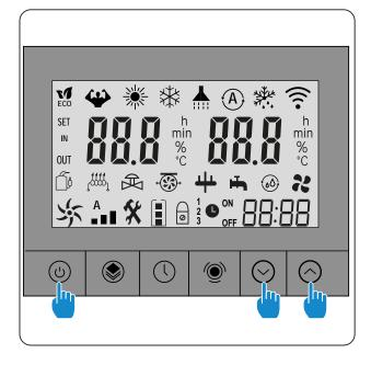
Press 0 + > + > simultaneously for 5s,  $\textcircled{$\widehat{\uparrow}$}$  flashes quickly, the control unit is ready to be paired.
