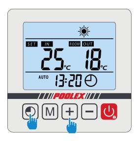
Press • + + simultaneously for 5s, see flashes quickly, the control box is ready to be paired.
