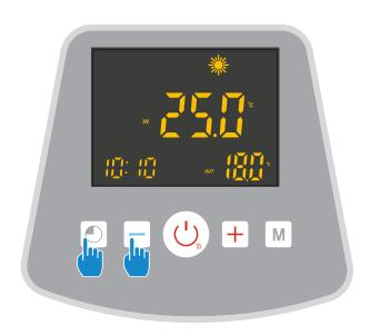
Press • + (b) simultaneously for 5s,  $\widehat{\ }$  flashes quickly, the control box is ready to be paired.
