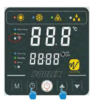
Press • + A simultaneously for 3s, • flashes quickly, the control box is ready to be paired.
