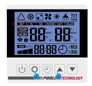
Press • + A simultaneously for 5s, set flashes quickly, the control box is ready to be paired.
