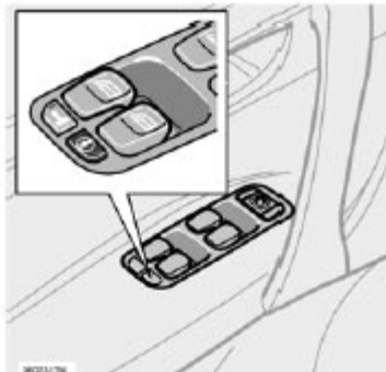
Cutout switch for rear windows
