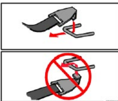
Fasten the attachment correctly to the ISOFIX lower anchors
