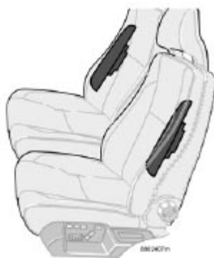
Location of the side impact (SIPS) airbag
