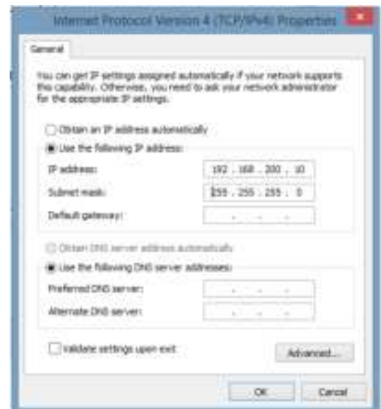
Fig. 2-14, Internet Protocol (TCP/IP) Properties Screen, Windows® 10
